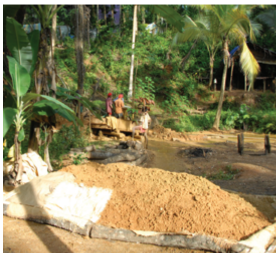
Fig. 9 (left). A pile of gem-bearing gravel washed from the illam and awaiting the second stage of washing.
