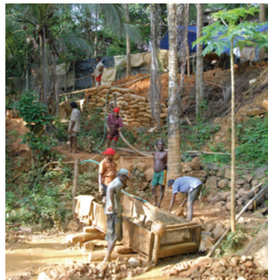
Fig. 7. The first-stage washing box for illam that has been extracted from the small shaft mine under the blue awning up the hill.
