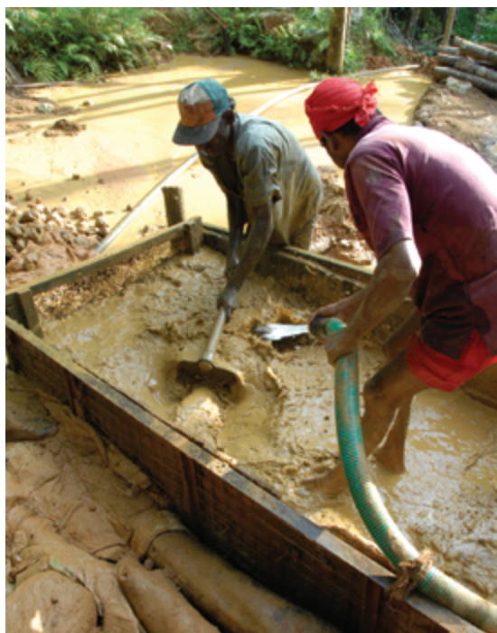
Fig. 8 (left). Washing the clay out of the illam with a powerful jet of water.
