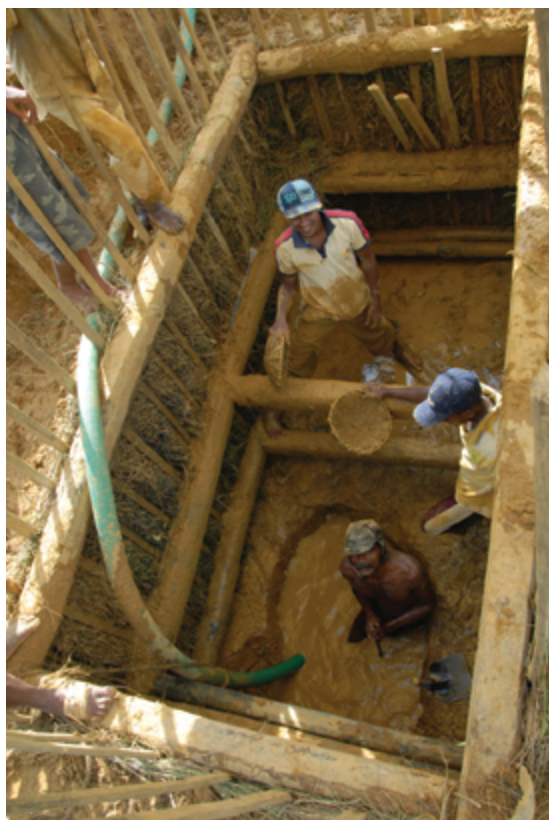
Fig. 5. Digging down to the gem-bearing illam in a small pit mine near Ratnapura.
